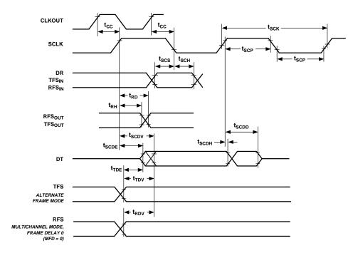
Figure 27. Serial Ports
